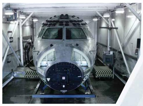
In our environmental chambers, our customers perform trials using temperatures between -55 °C and +85 °C. They are used to determine the optimal or critical conditions for the operating equipment, heating and defrosting systems and more to ensure the safety and comfort of drivers and their passengers.
